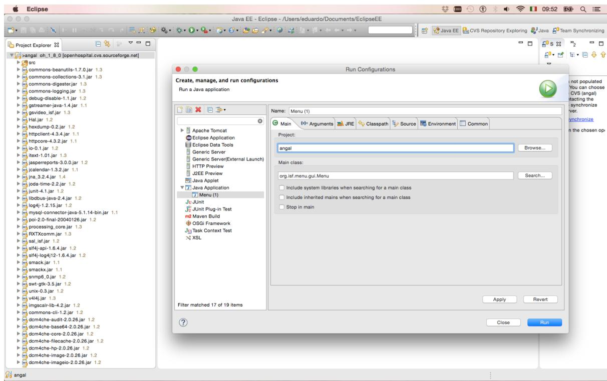
A “Run Configurations” window opens. Choose Java Application → <application’s name> - Menu (1) on this example. Select the “Main” tab, write “angal” on the “Project” field and check if the “Main class” is org.isf.menu.gui.Menu.
